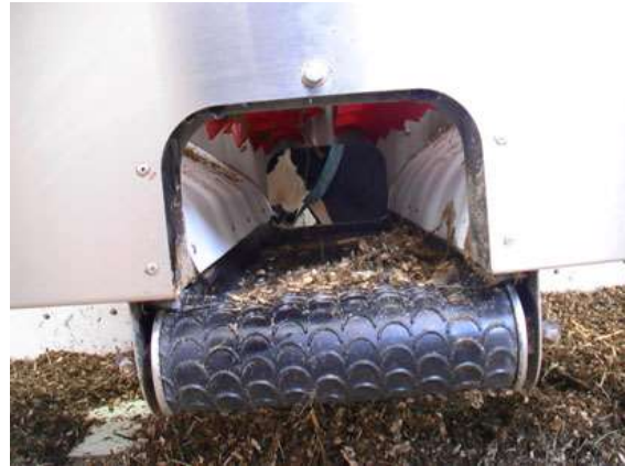
Slanted interior with calibrated conveyor deck for consistent distribution
